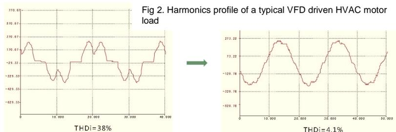
Fig 3. Harmonics current waveform distortion seen on typical 6-pulse VFD load before and after harmonics filtering
