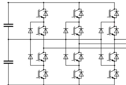
Fig 5. AHF and SVG are IGBT technology product designed to solve harmonics and PF swing problem in critical facility
