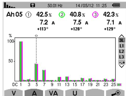
Fig 2. Harmonics profile of a typical VFD driven HVAC motor load
